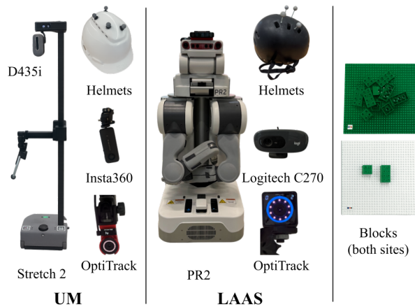
Fig. 5: Hardware used for the data collection.
