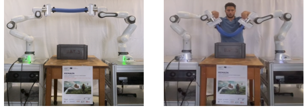
(a) Bi-manual manipulation of high stiffness foam. (b) Operator collecting data using kinesthetic guidance.
