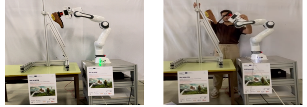
(a) FR3 grasping the shoe sole (b) Operator collecting data by attached to a rigid structure. kinesthetic guidance.
