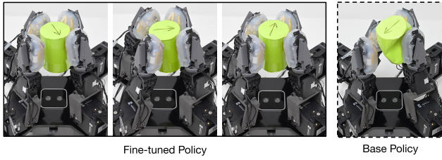
Fig. 7: Rollout of the fine-tuned policy at three time points. The base policy \pi_{\text{RL}}^0 = \pi_{\text{IL}} quickly crushes the paper object, while the fine-tuned policy using raw SpikeATac signals is capable of long rollouts without damaging the object.
