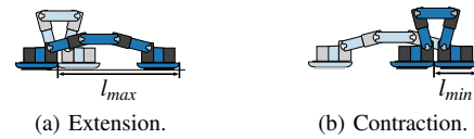
Fig. 2: Sliding gait phases for l_{\min}^{\text{sliding}} = 100 mm and l_{\max}^{\text{sliding}} = 290 mm.
