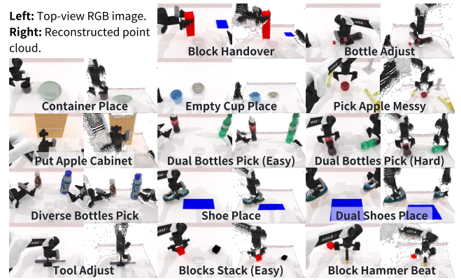
Fig. 3: Simulation benchmark – 14 bimanual manipulation tasks. Left: Top-view RGB image of the task. Right: Reconstructed point clouds via VGGT.
