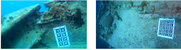
Fig. 4: The 4-by-2 and the 5-by-4 targets at Pamir wreck, which stayed at a fixed location for the Pamir1 and Pamir2 sessions.
