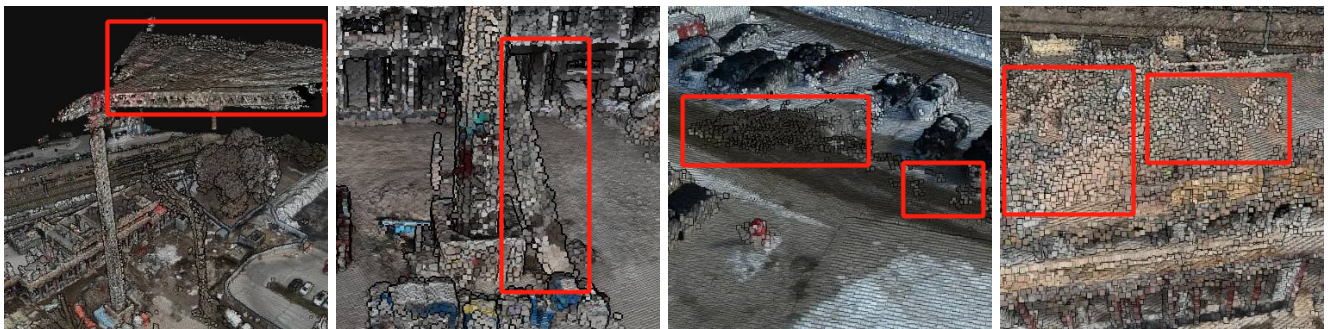
Fig. 6. Examples of dynamic elements in the construction site. Figures shown by DJI Modify to amplify the dynamic points. From left to right: moving crane, moving string attached to the crane, moving vehicle, and moving construction workers.
