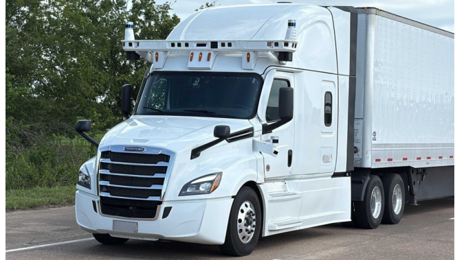
Fig. 1: Photo of autonomous truck. Designed for redundancy, the vehicle integrates four long-range 128-line spinning LiDARs (two on top, two on side panels), along with two IMUs and two VCUs installed inside the cabin.
