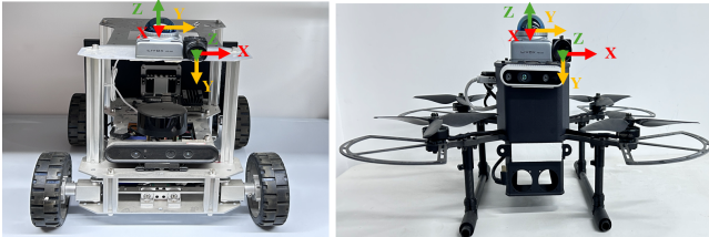
Fig. 4: Physical platform. The left side is the Livox MID-360 LiDAR, and the right side is the Prophesee EVK4-HD event camera. Data is collected using two mobile platforms: a ground-based mobile robot and an aerial drone.
