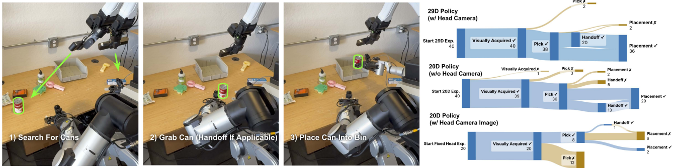
Fig. 4: Tabletop Task Rollout Sequence: (Left). The images show a real 29D policy evaluation rollout where the robot (1) scans for target cans across a cluttered workspace, (2) grasps the correct item with potential handoff between grippers, and (3) places it into the designated bin. (Right). The Sankey diagrams illustrate failure modes between policies with full 29D action space and active head-camera versus reduced 20D wrist camera-only and 20D + head-camera images baselines.
