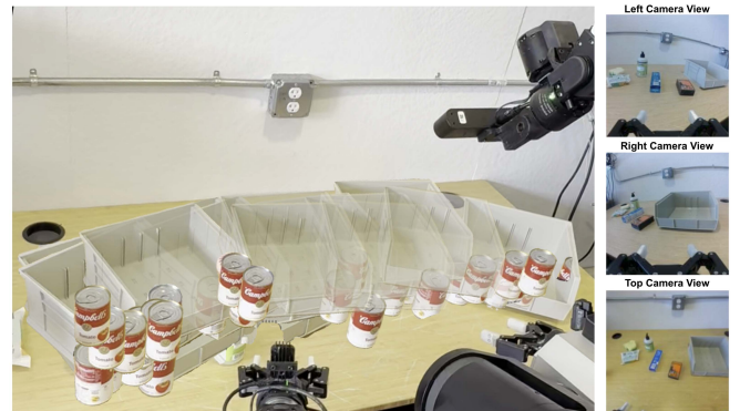
Fig. 5: Randomization distribution and example initial configuration of the tabletop environment highlighting the wide distribution of object positions and clutter scenarios used during evaluation rollouts. (Right). Initial configurations for target object may be outside of the immediate field of view of the initialized robot during experimentation. Target object and placement location may also reside on opposite ends of the workspace requiring a bi-manual handoff maneuver.
