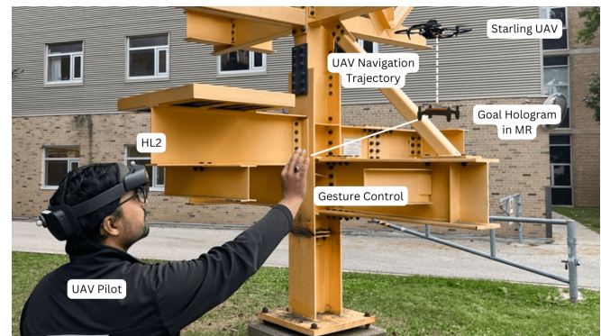
Fig. 5. UAV pilot using gesture control to set a goal pose in the MR App. The UAV autonomously navigates to the specified goal.
