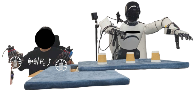
Fig. 1: The CDF-Glove and the whole machine teleoperation system. The CDF-Glove is worn on the operator’s hand to collect hand joint data and provide haptic feedback.
