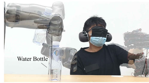
Fig. 11: Bottle grasping experiment based on haptic feedback.
