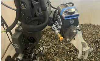
Fig. 3: An “opti-acoustic eye-in-hand” configuration is used to record the datasets. The sonar is mounted level relative to the manipulator’s wrist, and the camera is mounted 30 degrees off of vertical.
