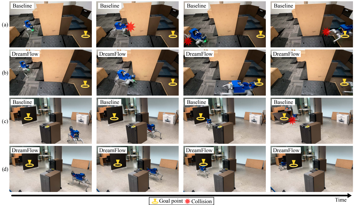
Fig. 6. Real-world navigation experiments on the quadruped robot, comparing baseline and DreamFlow. Time progresses from left to right across four snapshots. Yellow and red markers indicate goals and collision events, respectively. (a)–(b) Narrow environment with tight passages: the baseline policy frequently collides with walls at corners, whereas DreamFlow achieves collision-free navigation by anticipating corridor layouts beyond immediate perception. (c)–(d) Cluttered environment with box obstacles and a wall segment: the baseline collides with the wall due to limited perception, while DreamFlow successfully navigates without collisions through predictive terrain modeling.
