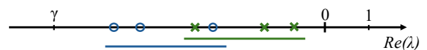
Fig. 2. Eigenvalue layout: slow system modes are shown in green and actuator modes in blue. The region left of \gamma \ll 0 indicates rapidly decaying modes that can safely be neglected. Spectral overlap of modes signals that neglecting actuator dynamics can induce significant modeling errors.
