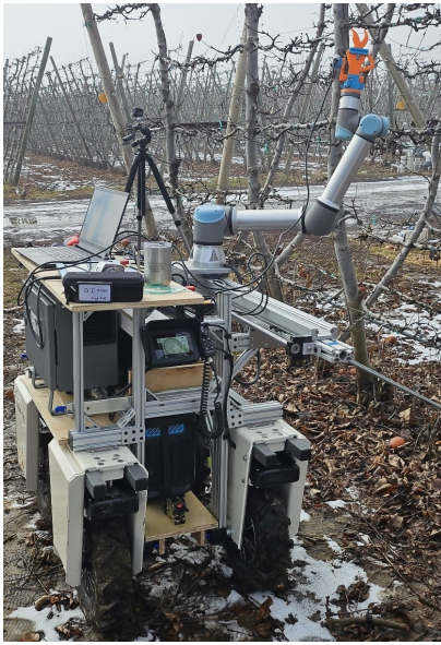
Fig. 2. Real world dormant tree pruning (Prosser, WA, USA; January 2025) with an industrial UR5e robot arm mounted to a ground robot. Baseline example of an agricultural task to guide robot arm optimization.
