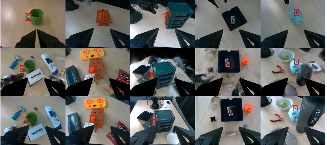
Fig. 3: Images of Optimal Views. Top row: demonstration optimal views. Middle row: test-time optimal views in 3DGS with gripper mask overlay. Bottom row: real world test-time optimal views. Red boxes indicate the task-relevant object parts. Test-time optimal views are derived by reconstructing the demonstration’s optimal viewpoints subject to minimal occlusion.
