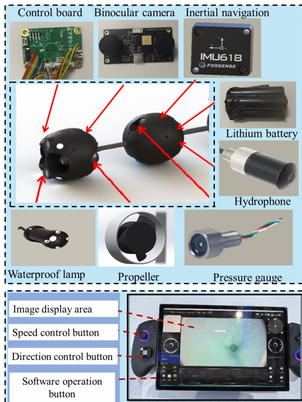
Fig. 11: Hardware and software system of pipeline robots
