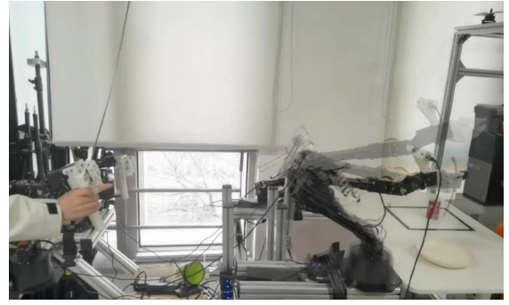
Fig. 6: Visualization of pronounced jitter in the baseline method, caused by the 20Hz joint replication process.
