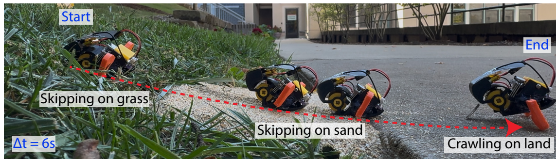
Fig. 9: Side-view sequences of TerraSkipper in outdoor tests. Panels show (left to right): skipping on grass, skipping on sand, and synchronous crawling on hard ground. Frames are overlaid every 6 s; each panel displays 6 s of motion.
