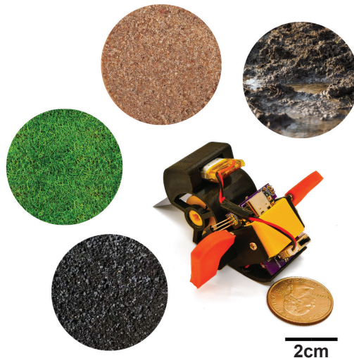
Fig. 1: TerraSkipper with representative challenging terrains shown in the surrounding circular pictures, on which the robot can locomote. A U.S. quarter and a ruler indicate scale.
