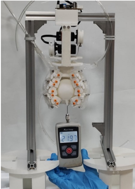
Fig. 9: Destructive testing of the proposed gripper to determine its maximum load capacity.
