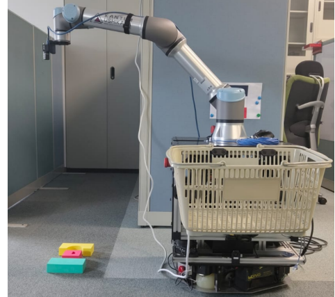
Fig. 2. Visual servoing setup: 6-DoF UR5 with wrist-mounted FLIR Blackfly S (eye-in-hand).
