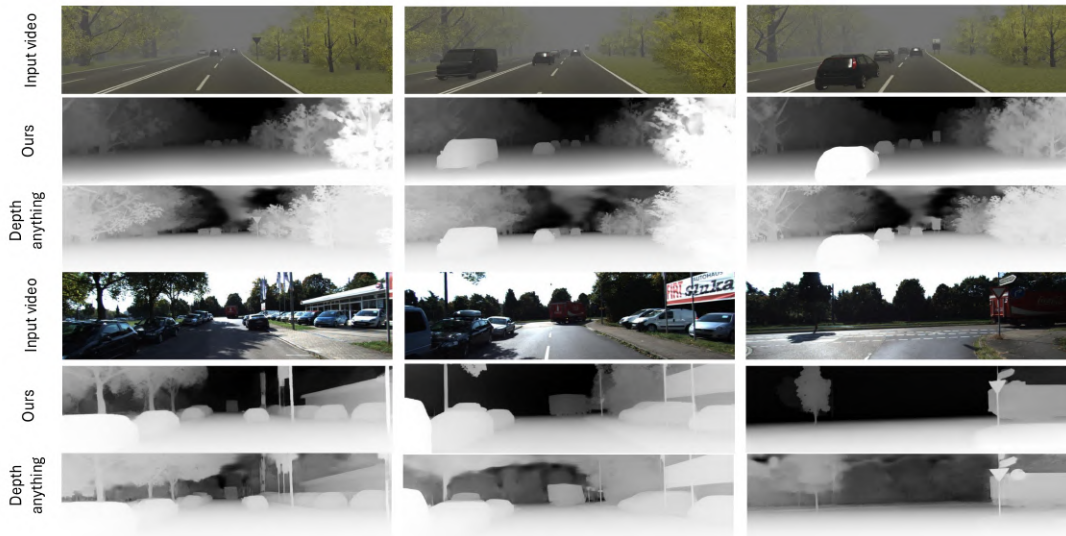
Fig. 4: Qualitative results comparison on VKITTI (top) and KITTI (bottom) . DepthAnything fails to recover fine object details in foggy weather and sky regions, our method estimates clearer and more temporally consistent depth.
