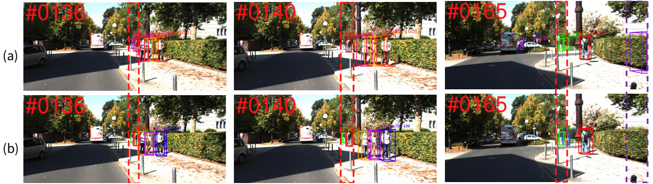
Fig. 2: Comparison of tracking performance on the KITTI dataset between the AB3D method (a) and our proposed method (b). Different colors correspond to distinct object identities. In sequence 18, AB3D demonstrates identity switches (a), while our method ensures continuous trajectory maintenance despite challenging conditions (b).
