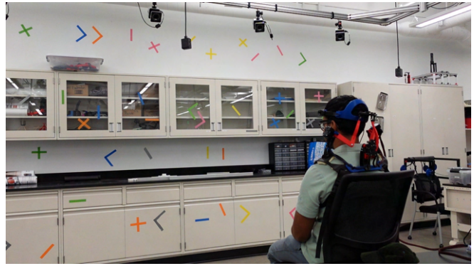
Fig. 8. A subject provides preference regarding eye tracking controllers applied to the Columbia Brace [30]. The eye tracking frame is placed over the subject’s glasses. The subject evaluated each controller by searching for a specific symbol and color combination on the wall. The clutter on the wall provides distraction to make the task more difficult and realistic.
