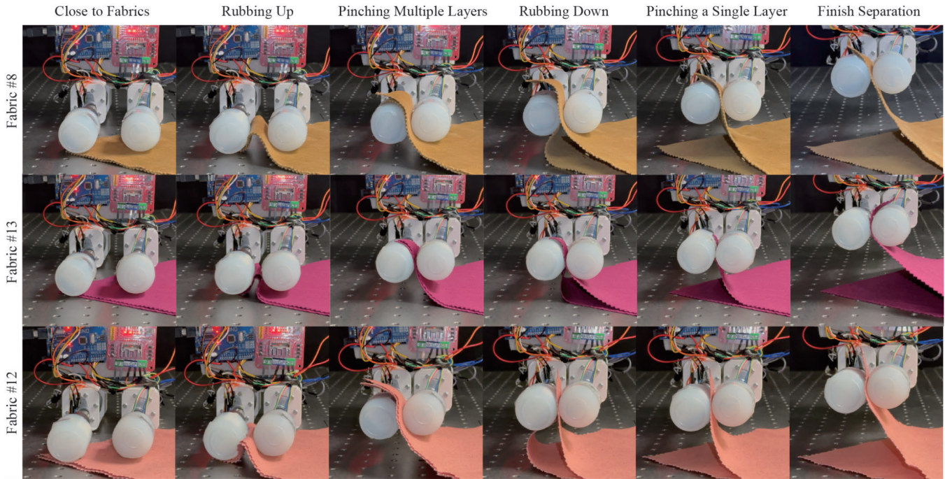
Fig. 7: The process of separating different fabrics using rubbing grippers.
