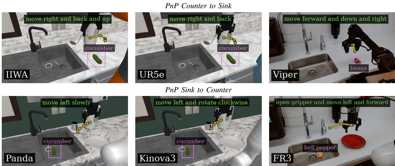
Fig. 6: We show examples of our real tasks (right) in comparison to their sim counterparts (left, middle). We also show actual predictions from Joint Reps models, which demonstrate similar predicted representations across different embodiments in unseen scenes.
