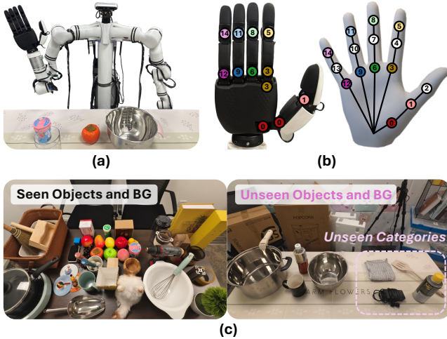
Fig. 5: (a) Robot setup. (b) Mapping between XHand and MANO, where joints sharing the same index indicate correspondence; white color denotes joints without counterparts. (c) Fine-tuning objects/environment and unseen objects/background for evaluation.
