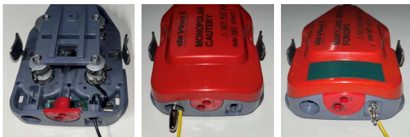
Fig. 3. Instrument wire connection. Non-polar instrument (left), monopolar (center), and bipolar (right). For non-polar instrument, the tool housing is opened and the wire insulation layer is removed for better visualization.
