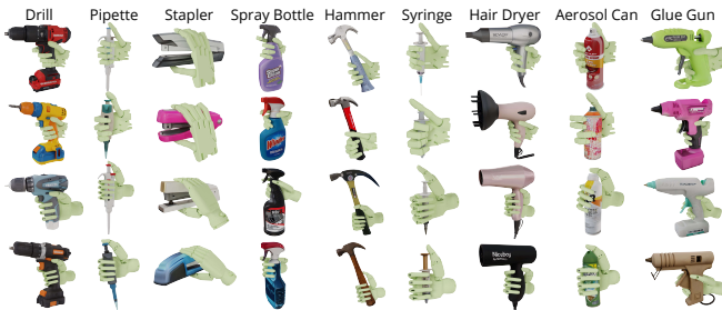
Fig. 4. Examples of generated data. We generate a functional dexterous grasp dataset consisting of 900 objects, 1.08 million images, and 11 million image–grasp pairs. The dataset spans across nine tasks and two different embodiments of different DoFs (Shadow and Inspire).
