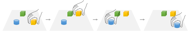
Fig. 1: Human demonstration of toy object manipulation. Humans can readily infer task procedures from a manipulation demonstration and express them in language (e.g., “pick up the yellow block” → “place it to the right of the green block” → “grasp the blue cylinder” → “put it on the bottom right of the table”). This linguistic description enables humans to accurately replicate the demonstrated action sequence.
