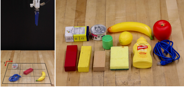
Fig. 6: Real robot experiment setup. (Left) The workspace is divided into a 3 \times 3 grid to provide an absolute spatial reference for task descriptions. A top-view image captured by an Intel RealSense D415 camera serves as the visual input to LACY. (Right) Objects used in the real-robot experiment, including both everyday items and selected YCB objects.
