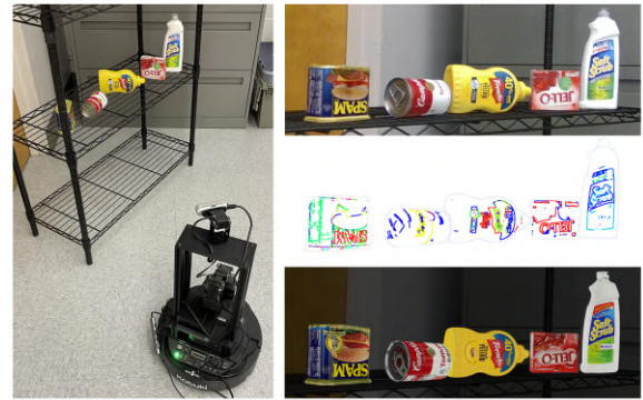
Fig. 8. Real-World Experiment. Left: experimental setup. Right (top to bottom): input scene, color-pair classification, and the final rendered pose estimate.
