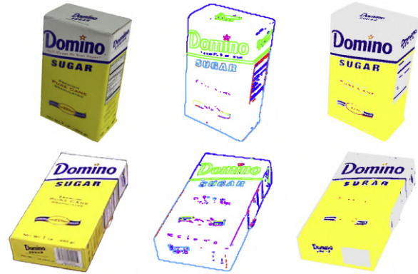
Fig. 1. Visualization of color-pair based classification. Left to right: input image, color-pairs visualized by class, and classified surface patches based on matching. Rows compare results on synthetic (rendered) vs. real (captured) images under varying illumination to demonstrate robustness.
