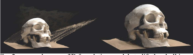
Fig. 2: we can leverage 3D foundation models to lift the skull image (shown in fig. 1) to a 3D point cloud (left), then leverage confidence estimates to further filter and clean the point cloud (right).
