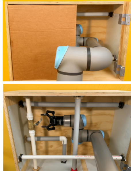
Fig. 1. A robot reaching a shutoff valve at the back of a cluttered cabinet. As visual sensing is occluded by the shelf door (top), the robot relies on contact feedback to navigate around obstacles.
