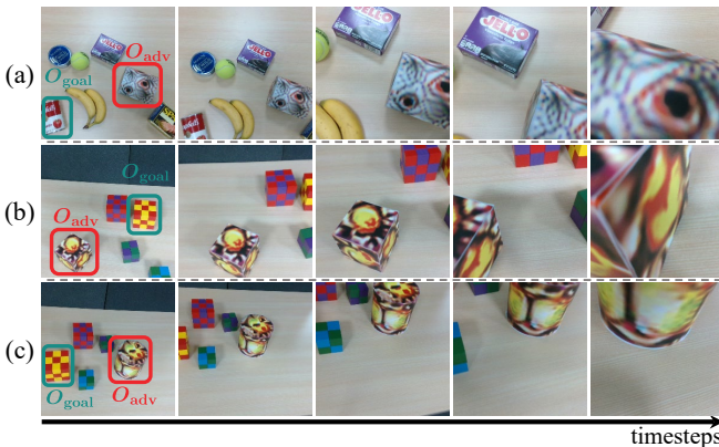
Fig. 8. Policy rollout with (a) a cylinder-shaped adversarial object in EnvA, (b) a cube-shaped adversarial object in EnvB, and (c) a cylinder-shaped adversarial object in EnvB.
