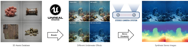
Fig. 3. Data synthesis pipeline. Unreal Engine 5 rendering pipeline for UW-StereoDepth-40K dataset.
