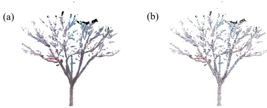
Fig. 3: Preprocessing of tree point cloud scanned from a RGB-D camera. (a) After removing noise and ground points; (b) After downsampling.
