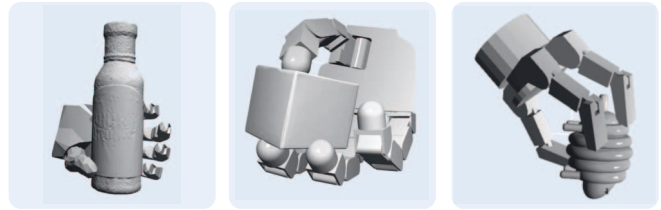
Fig. 1: Visualization of generated grasps on test unseen objects. Left: ShadowHand, Middle: Allegro, Right: Barrett
