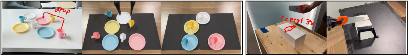
Fig. 11: Generalizing Cross-modal instructions to new setups, with the Place Cups task shown in the left and the Saw Block task on the right. An image with an instruction is overlaid, and we observe that the setups that the instructions are defined over are visually different from the execution setup, highlighting the generalization exhibited. We can also provide instructions such as “repeat 3x”.
