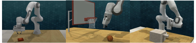
Fig. 9: Without hierarchical precision coupling, directly seeking the VLM reasoning model to provide trajectories often leads to the robot not adequately reaching the object that we need to interact with, such as the button, basketball and Jenga block.
