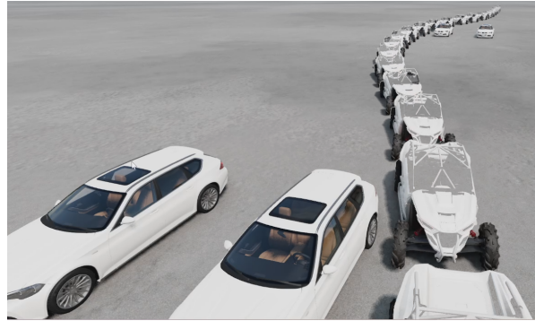
Fig. 1: Tracking of high-speed emergency collision avoidance trajectories in BeamNG simulation. Video available at https://tinyurl.com/trajopt
