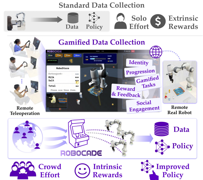
Fig. 1: We develop RoboCade , a platform that gamifies the collection of robot demonstration datasets. In standard data collection approaches ( top ), hired operators or researchers collect demonstrations using in-person teleoperation, which requires access to a robot and can be tedious and time-consuming. RoboCade ( bottom ) is a remote data collection platform that integrates gamification into both system and task design, making robot data collection more engaging and accessible to a broader set of users.
