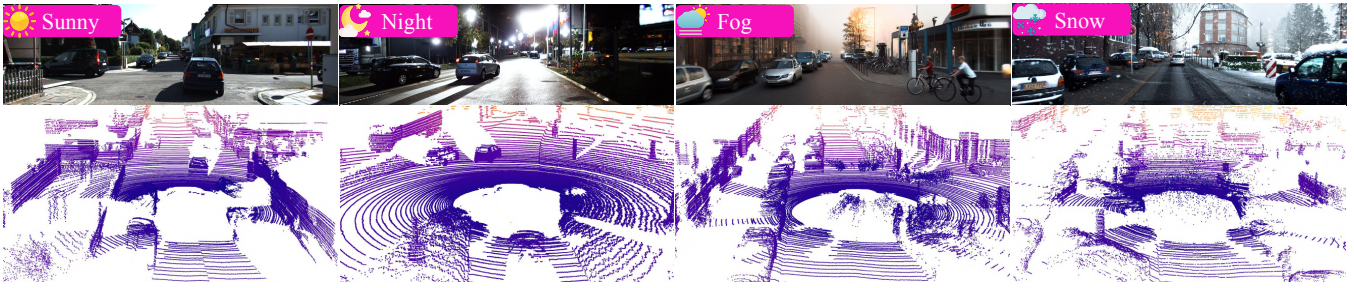
Fig. 1. Motivation for Veila . The top row shows monocular RGB images used as conditions under various weather settings (sunny, night, fog, snow). The bottom row presents panoramic LiDAR scans generated by our framework, enabling controllable high-fidelity cross-weather synthesis.
