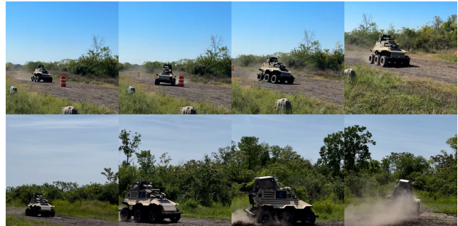
Fig. 1: Autonomous vehicle avoiding obstacles (top) and taking corners at speed (bottom) controlled using TADPO-trained end-to-end policies.
