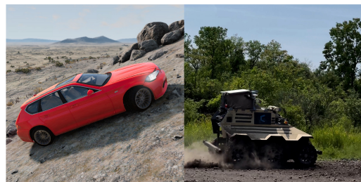
Fig. 5: A comparison of the training vehicle in simulation environment and the deployment vehicle in deployed environment. A large embodiment gap can be observed both vehicle dynamics and the terrains.
