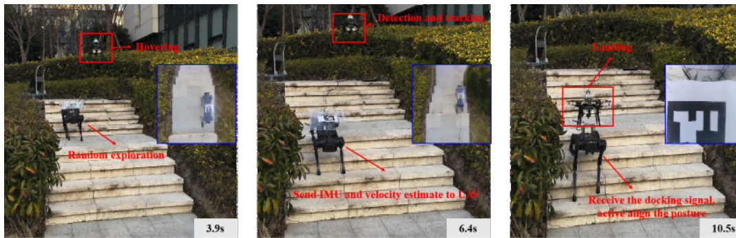
Fig. 8. The docking experiment in an outdoor 17 cm staircase scenario is presented. Two camera perspectives are showcased in this demonstration. The Top view represents footage captured by an external fixed camera, while the Bottom view displays the perspective from the onboard monocular camera located at the underside of the UAV.
