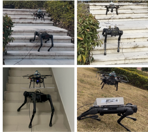
Fig. 1. Docking experiments in complex terrains. The top-left and top-right show tests on a 17 cm outdoor stair where the quadruped actively adjusts its posture while ascending and descending. The bottom-left shows an indoor 15 cm stair experiment, and the bottom-right presents docking on a 30° outdoor rough slope, demonstrating the robustness of the proposed method.
