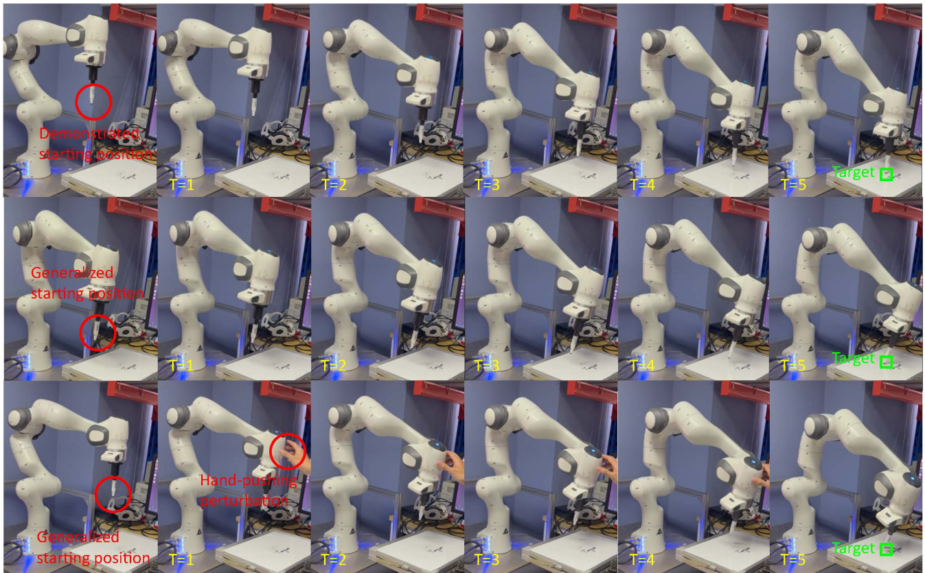
Fig. 7. Experimental validation of learned reaching dynamics on a Franka Emika robotic arm. Row 1: Reproduction of the demonstrated trajectory. Row 2: Generalized convergence from a new initial position. Row 3: Perturbation recovery through hand interaction. The experiment demonstrates the system’s inherent stability and disturbance rejection capabilities.
