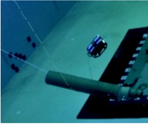
Fig. 6: During the experiment, the ROV became entangled with the pipe, illustrating a typical CPP entanglement.
