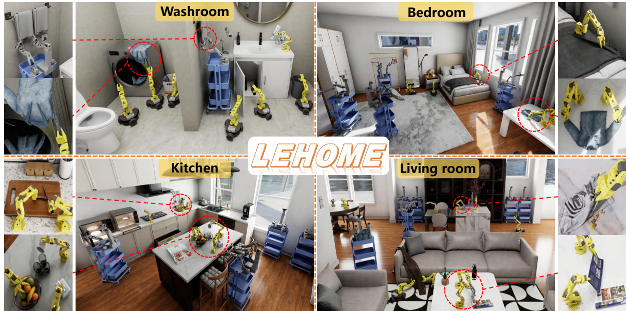
Fig. 1: LeHome provides a high-fidelity simulation platform by integrating various household scenarios and various objects within the scenarios, especially deformable objects.
