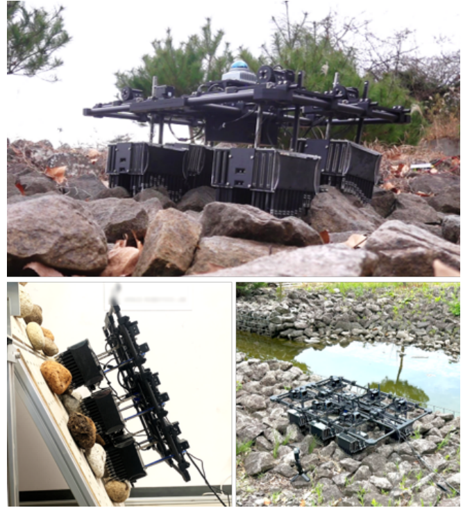
Fig. 1. The pin-array unit passively adapts to irregular terrain shapes, enabling stable ground-gripping locomotion (top). The robot demonstrated stable adhesion performance on steeply inclined rocky terrain (bottom left) and was also deployed in a natural rough landscape (bottom right).
