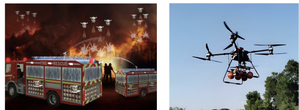
Fig. 1. Multi-drones system and fire base stations working together in firefighting (left) and a drone deploying firefighting bombs (right).
