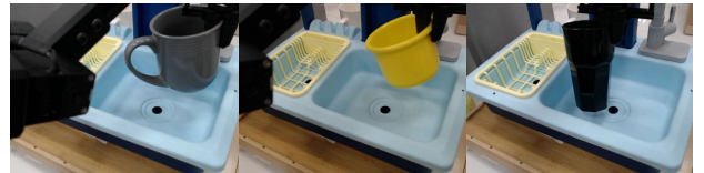
Fig. 7: Successful lifts on real robot. OpenVLA-FT succeeds at lifting cups of varied shapes, textures and sizes.
